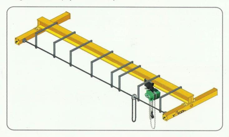
Our premium quality HOT cranes are available with 100% radiography welded joints of bridge and end carriage. Our material handling cranes comply with ISS: 2261 or ISS: 2062 which ensures resistance to vibrations. The wheel assemblies of the crane are heat treated to achieve a special sorbatized structure up to a depth of 15-20 mm from the surface.
